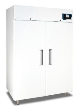
The handles are flush-fitting type so do not increase the size of the refrigerator. The doors are also fitted with a spring loaded automatic closing devices for openings inferior 90° and special door switches that stop the internal ventilation at the door opening (to limit the air cold loss) and light the internal lighting at every opening
